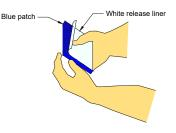
3- Remove VISCOTAQ<sup>®</sup> Coating Patch from packaging and peel off release liner.
