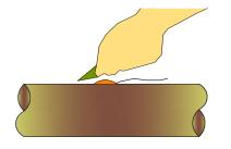
1- Use Abrasive Cleaning Pad included in kit if needed to clean exothermic weld and existing coating around the weld where patch is to be applied.
